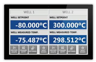
Clear, large-digit home screen displays current well temp. and setpoint(s) and gives users **ONE TOUCH** access to controls
